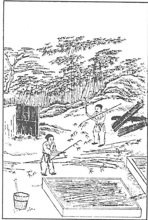
Cut bamboo is washed and steeped in a water pit to prepare material for making paper.
